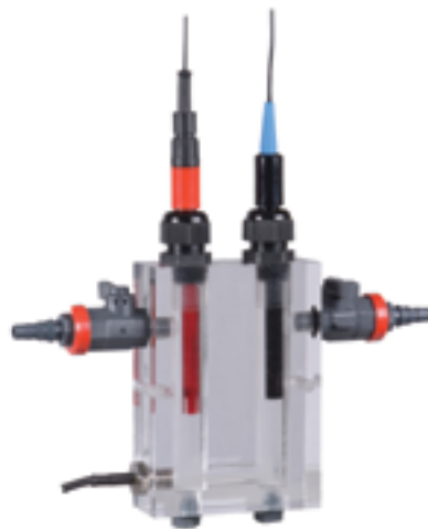
FC3020T flowcell with integrated T sensor
