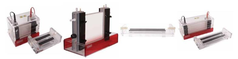
Our EVS3xxx vertical systems allow for fine resolution of protein or nucleic acid fragments on one or two acrylamide gels (PAGE). PAGE separation offers the superior resolution necessary to separate native or denatured proteins and nucleic acids in applications such as SSCP or dinucleotide repeat analysis using western blotting and also for automated protein sequencing analysis.
