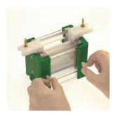
Fully tighten the screw for the Mini vertical and the screws sequentially and in an even manner for
