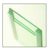
**Note**: The glass plates with bonded spacers have an arrow in the top of the spacers which are slightly longer than the glass plate to indicate the top.
