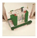
• With the cam pin handles facing directly downwards, turn the cam pins fully through 180° or until the insert has tightened onto the silicone mat.
