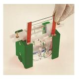
The Slab Gel Insert contains pressure bars which impart even pressure onto the glass plates and allow even screw pressure transfer onto the sealing edge of the glass plate, ensuring complete sealing.
