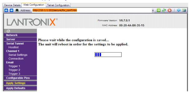
When finished, the <u>Home</u> screen will reappear. To see the new configuration, it is best to close the Device Installer program and restart it.
