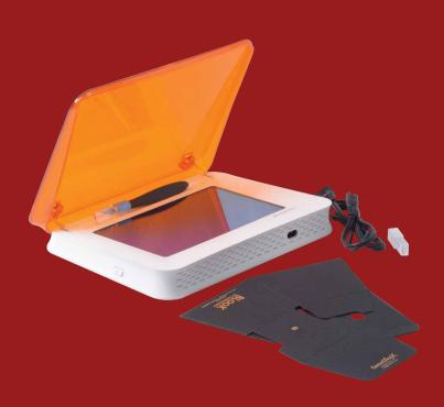
BLooK is a remarkable blue light LED transilluminator for the detection of nucleic acids or protein under non-UV conditions. The wavelength of the special blue LED lights is 470 nm, hence no damage to your nucleic acids or protein. Also, since UV is not used, there is no need for any special personal eye or skin protection.
