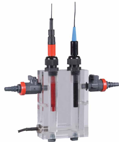
FC3020T flowcell with integrated T sensor
